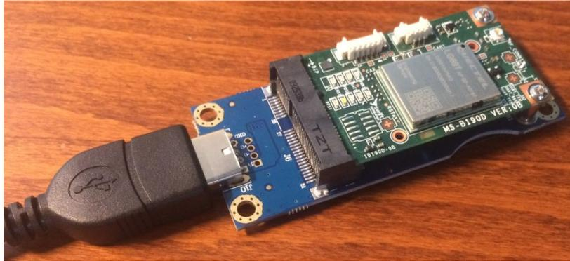
Fig 2. PGM on the USB Adapter Board
