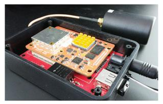
Piksi Multi is a multi-band, multi-constellation real-time kinematics (RTK) GNSS receiver that provides centimeter-level accuracy at an affordable cost. Being multi-band means fast convergence times measured in seconds, not minutes. Access to multiple satellite constellations improves availability, reliability and range between base and UAS.
