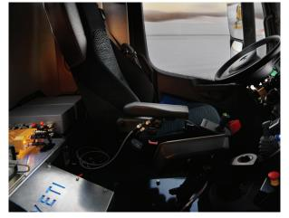
To solve the heading problem, Yeti implemented a second Swift receiver. Piksi Multi was added with antennas placed within approximately 2 meters distance on the cabin. As the general movement of the cabin is perpendicular to the direction of vehicle movement, the movement of the cabin still influenced the vehicle's position measurement but the heading information became centimeter-accurate and stable from this point on.
