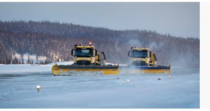
Swift Navigation's RTK GNSS technology provided the centimeterlevel accurate positioning and heading control required for Yeti's snow plows to drive together to autonomously clear airport runways.
