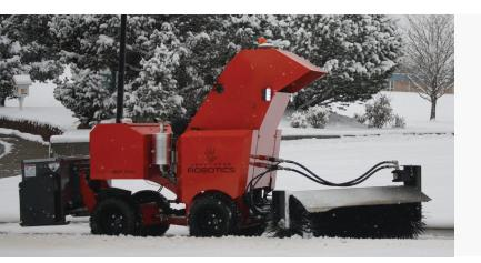
The highly-accurate Piksi Multi and Duro RTK GNSS receivers make it possible for our SnowBot Pro to navigate autonomously and accurately.
