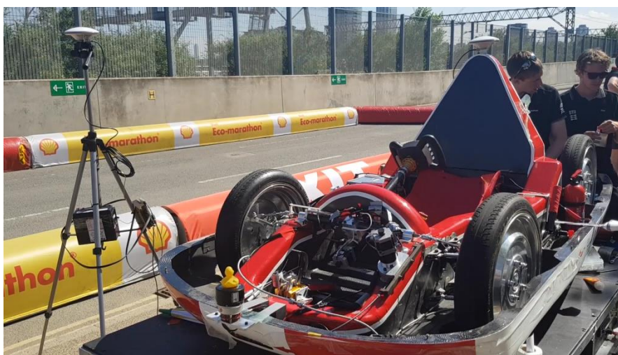
Figure 8: RTK base station and DTU Dynamo without top shell
