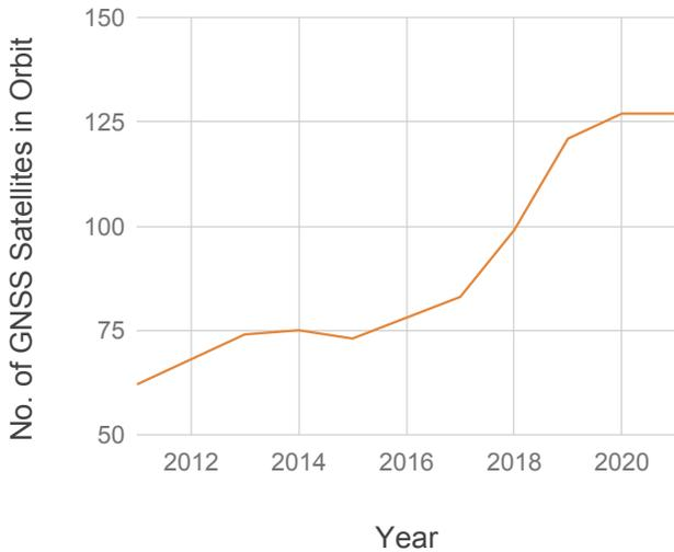
Fig. 3. Number of GNSS satellites in orbit as a function of time. Between 2017 and 2020, China’s BeiDou constellation and the E.U.’s Galileo constellation became operational, adding over 40 navigation satellites available to end-users. Today modern multi-constellation GNSS receivers have access to 125 satellites, while in 2005, GPS-only receivers could use less than 30.
