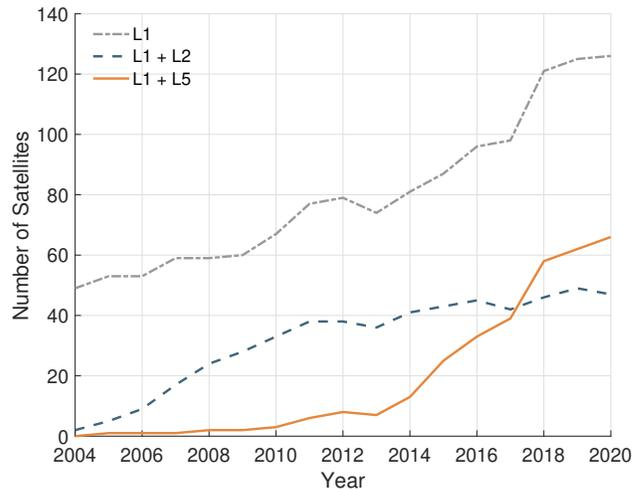
Fig. 5. Number of GNSS satellites with L1 (E1, B1C), L2, and L5 (E5a, B2a) civil signals as function of time.
