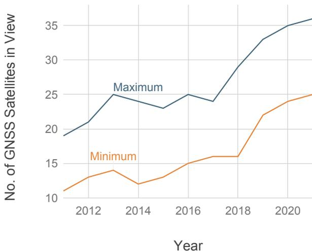
Fig. 4. Number of GNSS Satellites visible in San Francisco, CA over a 24 hour period. By 2020, there is always more than 25 satellites visible for navigation. Four satellites is sufficient for determining position. The additional satellites increases accuracy, enable fault detection and exclusion between satellites and constellations, and expands GNSS coverage into areas with significant sky occlusion.
