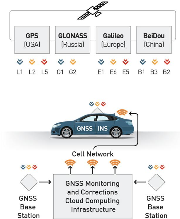
Fig. 2. The modern GNSS automotive ecosystem. Vehicles equipped with automotive-grade low CSWaP hardware receives signals from four satellite constellations across three frequency bands. A sparse ground station network backed by cloud computing provide error corrections and fault monitoring, delivered using standardized protocols via cellular networks.
